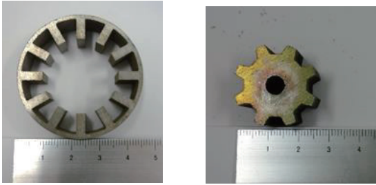
Fig. 8 Stator and rotor cores of SMC-based SR motor manufactured by using wire electric discharge machining.
