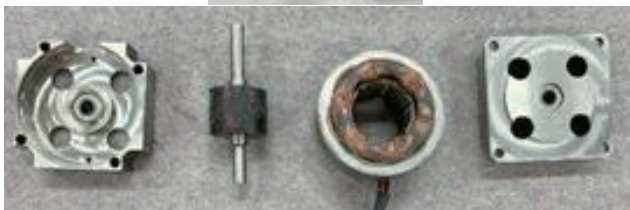
Fig. 3 Appearance of the prototype surface-mounted PMSM (top) and its parts disassembled (bottom).
