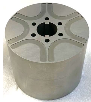
Fig. 2 Injection molded Sm-Fe-N bonded magnet IPMSM rotor. (Φ 60-L50mm)
