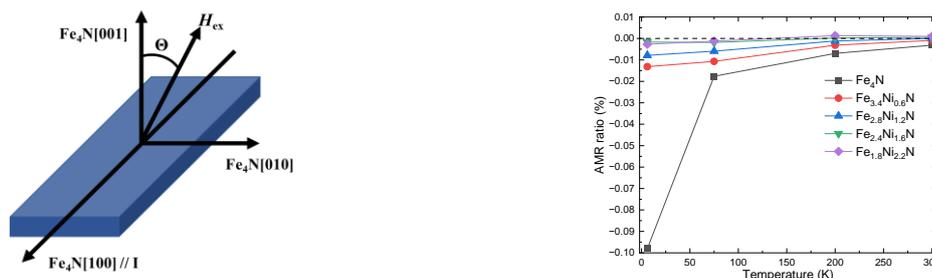
Fig. 1 A schematic geometry of the transverse AMR measurement. Fig. 2 Temperature dependance of AMR ratio of  $\text{Fe}_{4-x}\text{Ni}_x\text{N}$  films.
