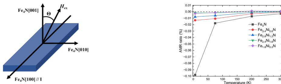
Fig. 1 A schematic geometry of the transverse AMR measurement. Fig. 2 Temperature dependence of AMR ratio of \text{Fe}_{4-x}\text{Ni}_x\text{N} films.
