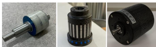
(a) Inner rotor (b) Pole-pieces (c) Magnetic gear Fig. 3 Appearance of the prototype magnetic gear.
