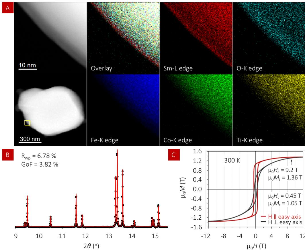
Fig. 1 Structural analysis and magnetic properties of chemically synthesized Sm(Fe<sub>0.8</sub>Co<sub>0.2</sub>)<sub>11</sub>Ti@Sm core@shell mesoscopic particles: (A) HAADF and EDS elemental mapping image, (B) Rietveld refinement synchrotron XRD pattern, and (C) M–H curves.
