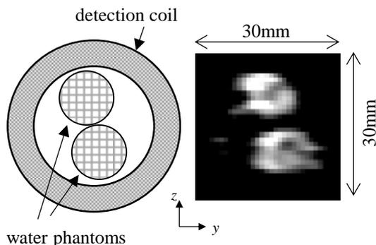
Fig. 1 Magnetic resonance image of water phantoms taken by the detection coil at 70  $\mu\text{T}$ .
