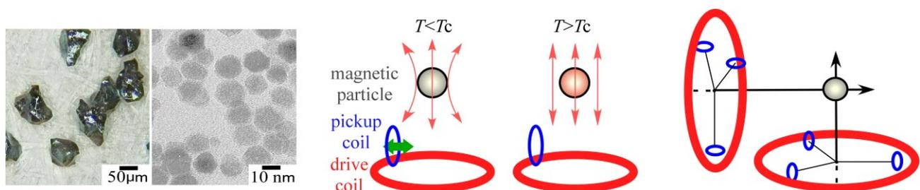
Fig. 1 Heating elements (microsize ferromagnetic implant with low Curie temperature and magnetite nanoparticles) (left), the concepts of wireless temperature measurement method (middle) and localization method (right) for the implant using the voltages induced in pickup coils around its Curie point.
