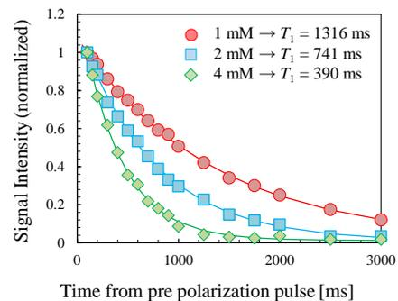
Fig. 2 Measured relaxation curves and calculated relaxation time of  $\text{NiCl}_2$  aqueous solution phantoms.
