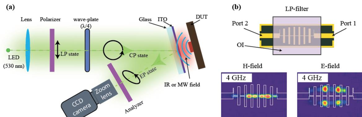
**Figure 1.** (a) Illustration of measurement principle of the TEOIM system. (b) The top shows the schematic of the tested lowpass filter and the optical indicator. The bottom images depict the visualized microwave H-field and E-field distribution images of the DUT at 4 GHz.
