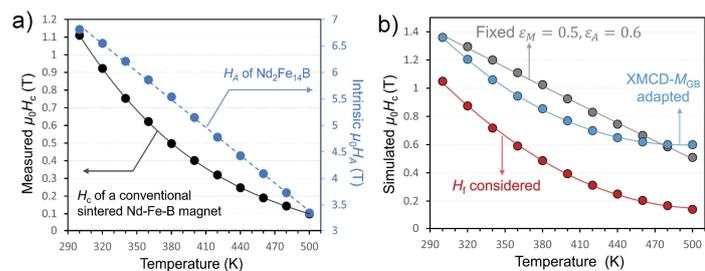
Fig. 1 (a) Comparison of the temperature dependence of coercivity of conventional Nd-Fe-B sintered magnet and intrinsic anisotropy field of Nd<sub>2</sub>Fe<sub>14</sub>B [6]. (b) Simulated temperature dependence of coercivity when grain boundary is ferromagnetic with and without consideration of temperature dependence of  $M_s^{GB}$ ,  $A^{GB}$ , and thermal activation [6].
